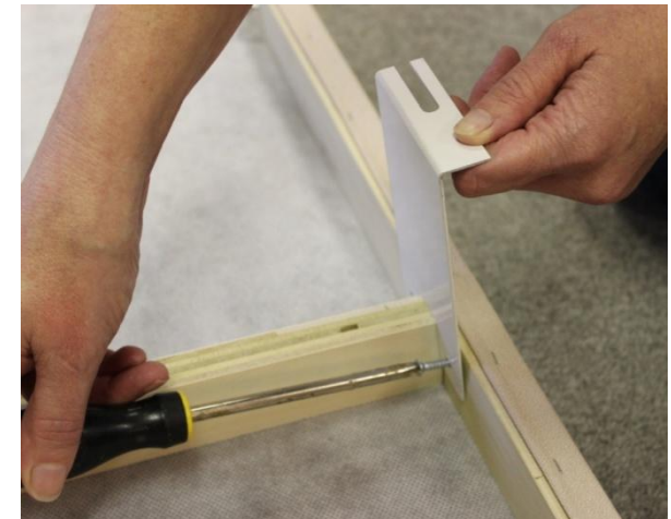
Using wood screws, attach each bracket to frame straddling the center support
